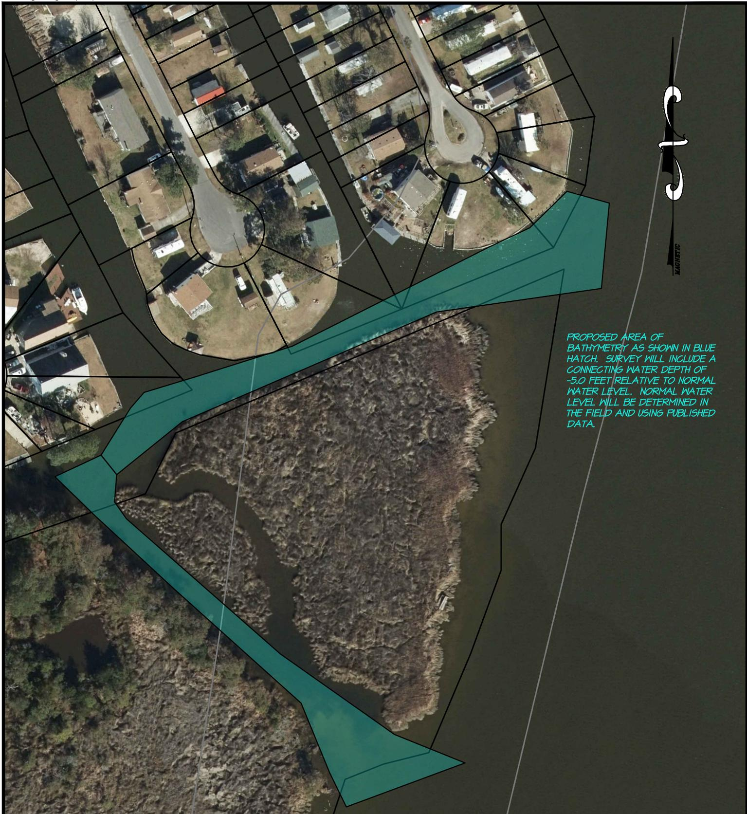
PROPOSED AREA OF BATHYMETRY AS SHOWN IN BLUE HATCH. SURVEY WILL INCLUDE A CONNECTING WATER DEPTH OF -5.0 FEET RELATIVE TO NORMAL WATER LEVEL. NORMAL WATER LEVEL WILL BE DETERMINED IN THE FIELD AND USING PUBLISHED DATA.
